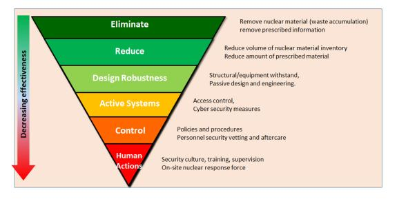
Figure 4 Illustrative secure by design hierarchy of controls.
