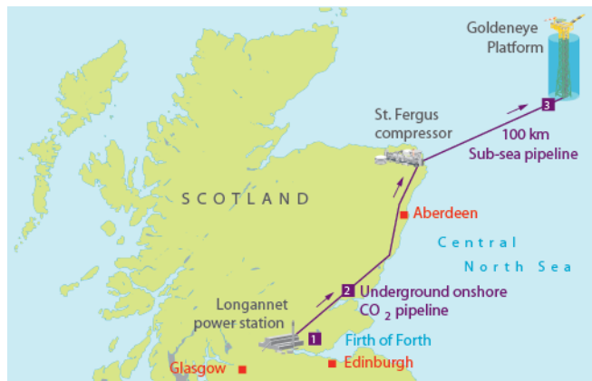
Fig 1. The Longannet to Goldeneye CO 2 capture, transport and storage scheme
