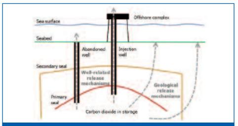
Fig. 2 - Carbon dioxide release mechanisms from offshore underground storage
