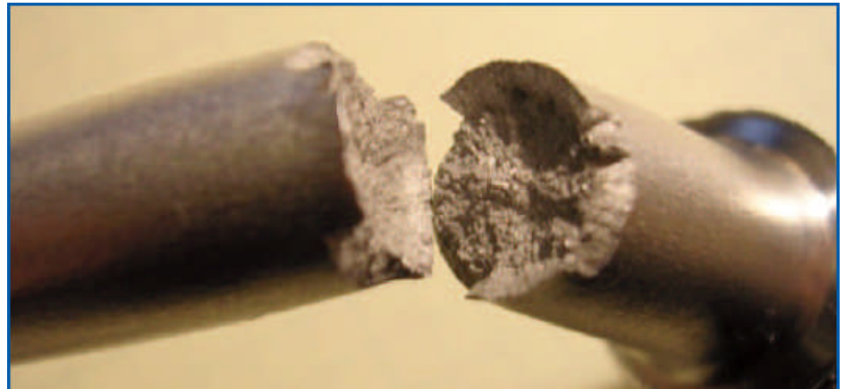
In tensile testing, samples are deliberately tested to destruction to characterise a material's ultimate strength. This principle is scaled up for 'stress testing'.
